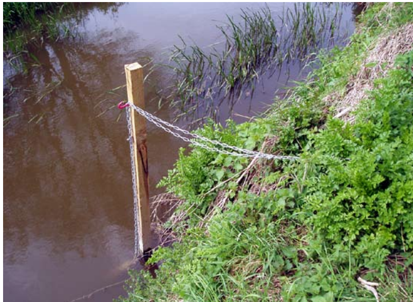
A YSI water quality sonde is suspended in the River Eden to monitor water levels as some water is removed to replenish Bough Beech Reservoir.
